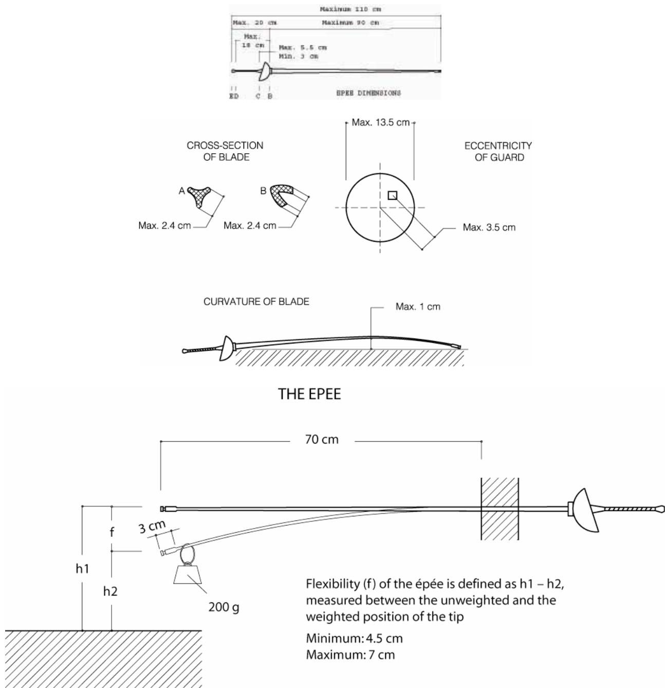
**Figure 9. Epee dimensions and flexibility**
