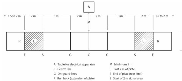
For foil and épée the conductive surface must cover the whole of the length and breadth of the piste, including its extensions (run back) (cf. Article T.13s, m.57)
